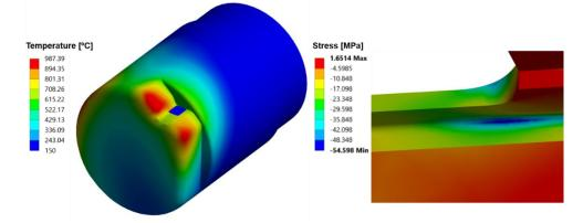
Figure 1 a) Probe head temperature distribution and b) inner probe head slot mechanical stress at the end of a simulated 4 second plasma discharge
