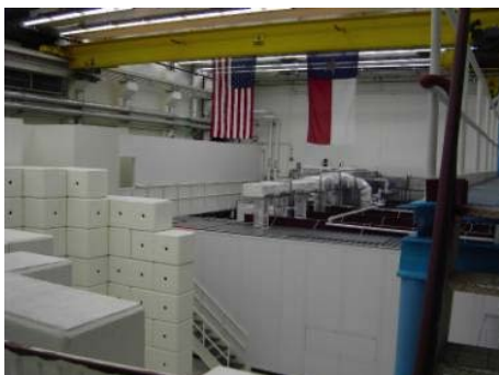
The Texas PW laser bay, with the radioactive shielding at first plane.
