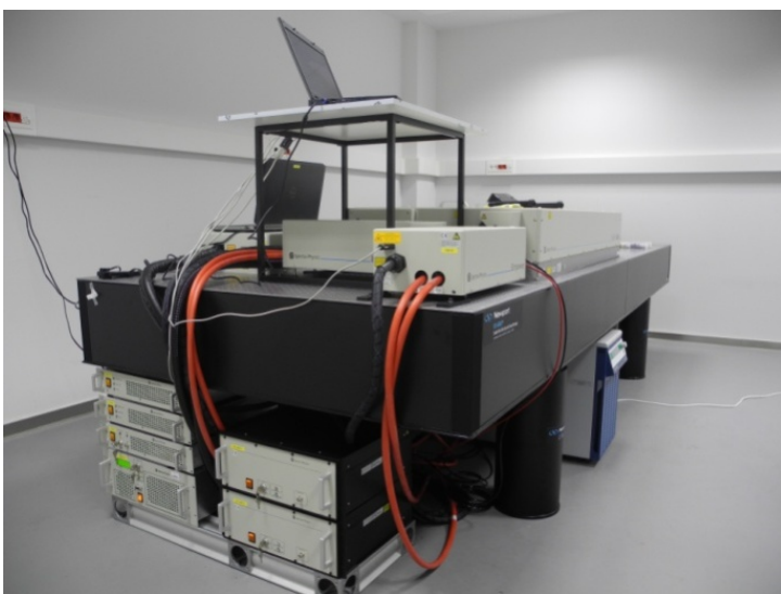
View of the femtosecond CPA Ti:Sapphire laser system with kHz repetition rate (HRR)
