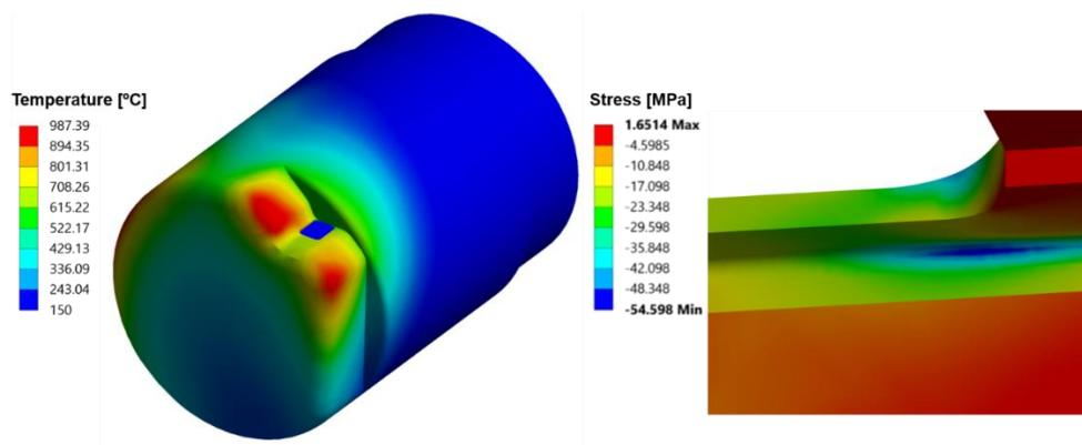
Figure 1 a) Probe head temperature distribution and b) inner probe head slot mechanical stress at the end of a simulated 4 second plasma discharge
